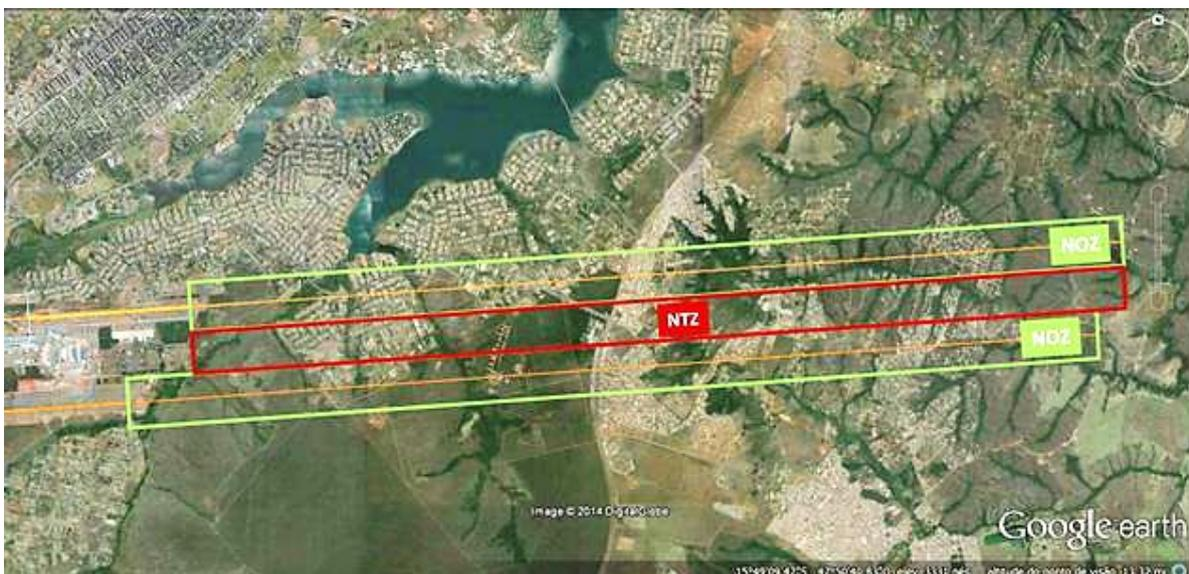
Figure 1: NTZ and NOZ configuration of SBBR runways 29
